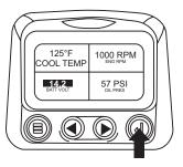
9. The parameter that is highlighted is the selected parameter for the screen. Use the "Arrow Buttons" to highlight the new parameter to be placed in the quadrant selected in the previous screen.
